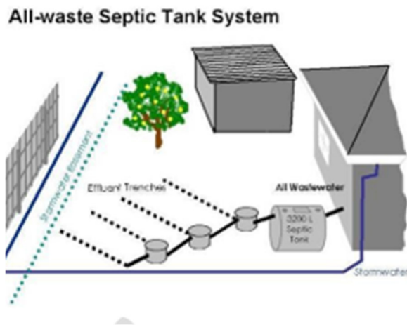
Figure 1: A typical septic tank system installation
