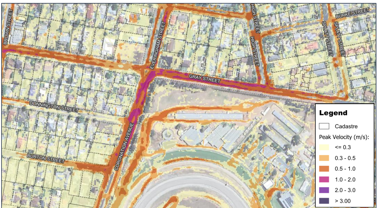
Figure 5-37 Peak Velocity on the Overland Flow Path on Gray Street and Coronation Avenue in the 1% AEP Event
